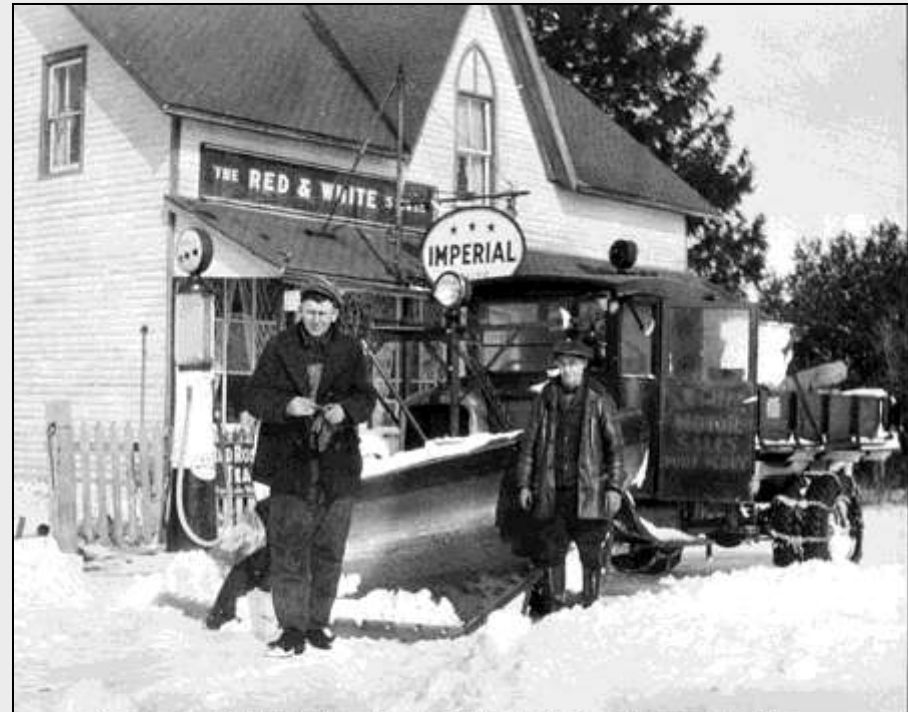
The first snowplow to be operated in Ontario County was owned by Harold Archer of Archer Motors, Port Perry. The snowplow is seen here sitting in front of the Scugog Island "Red & White" store in February 1939. Note the big 'V' shaped plow on the front of the truck, with dual-chained wheels on the rear. Pictured beside the truck are, left, Ross Prentice and at right, Don Anderson.
